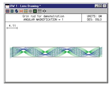
The drawing above shows both on-axis and off axis beams. Note that the off-axis beam for both the upper and lower rim rays is truncated by the edge of the rod. In order for this to happen, you must turn on the Aperture check all GRIN segs general operating condition. If you don't, the rays will be free to propagate outside the boundary defined by the aperture on the surface for with the GRIN material is defined.
